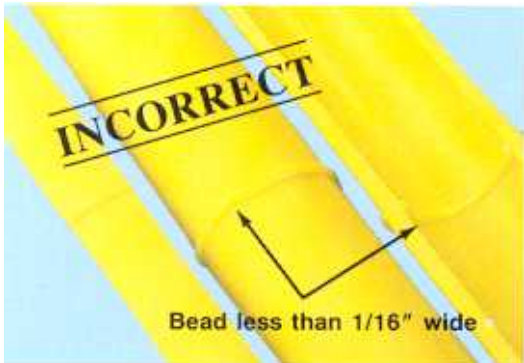
(FIGURE 26) MELT BEAD TOO SMALL
