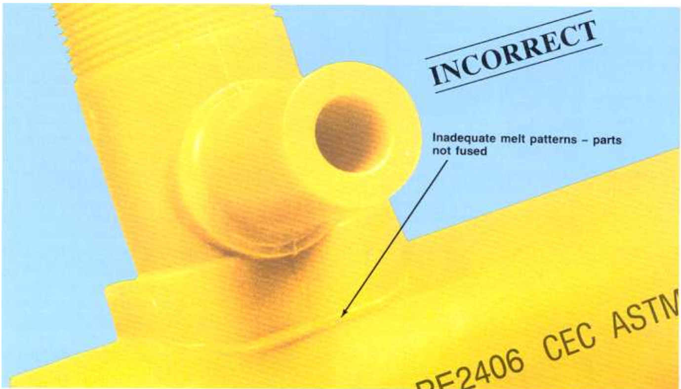
(FIGURE 11) COLD FUSION — EXCESSIVE COOLING BEFORE JOINING
