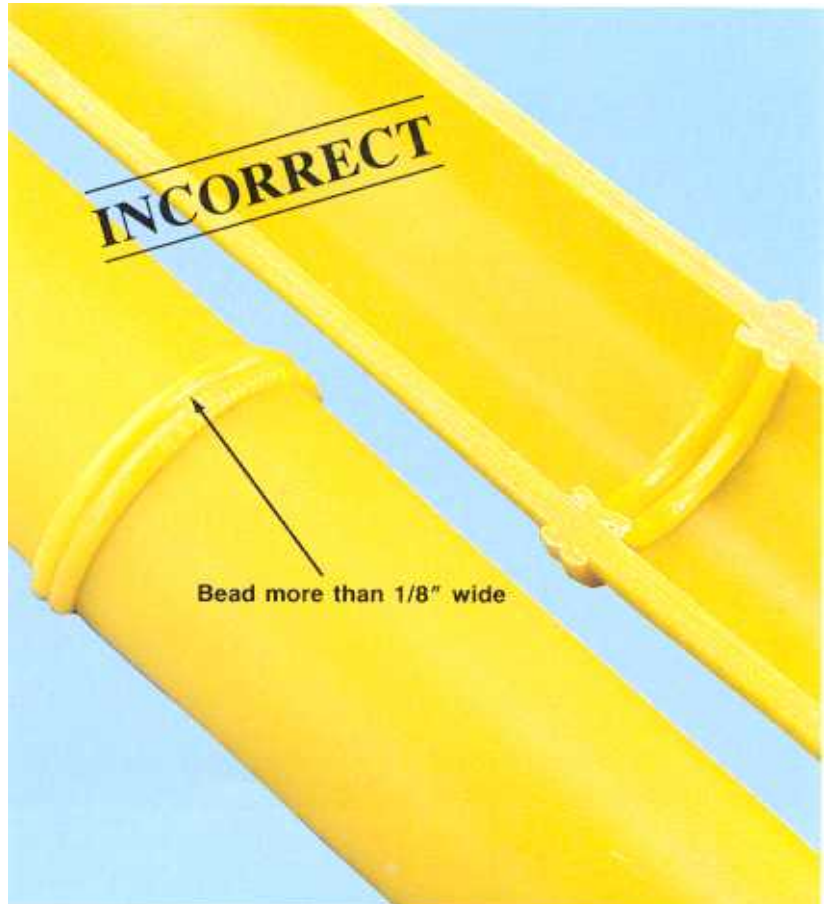
(FIGURE 28) MELT BEAD TOO LARGE
