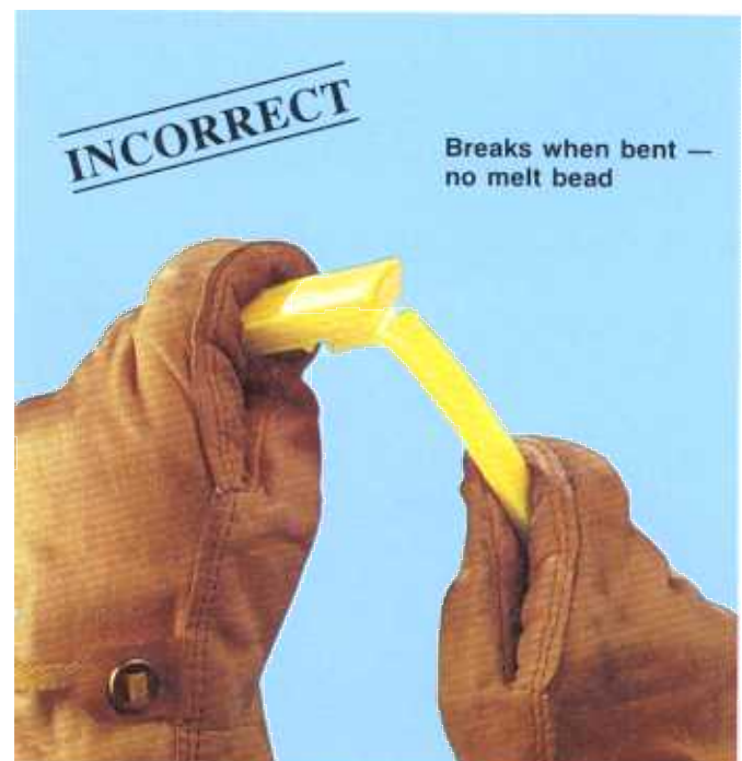
(FIGURE 7) MELT RUBBED OFF WHEN REMOVING HEATER
