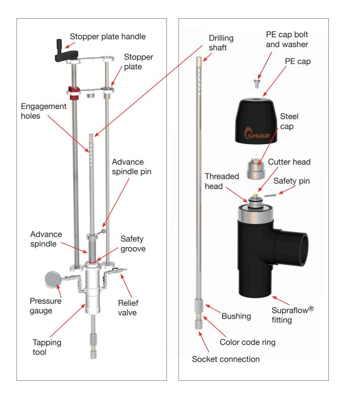
A branch saddle compliant with Supraflow<sup>®</sup> fitting instructions must be used. Ensure that the branch saddle is fused to the main according to manufacturer's recommendations and industry standards. Fuse the Supraflow<sup>®</sup> Gas Tap to the branch saddle.
