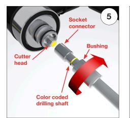
DRILLING SHAFT ATTACHMENT Attach drilling shaft socket connector to cutter head, slide bushing over socket connector, and ROTATE bushing (clockwise) by hand, until it bottoms out. Pull drilling shaft to check it is correctly engaged.
