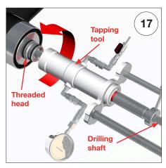
TAPPING TOOL REMOVAL Rotate tapping tool (counterclockwise) until released from threaded head and slide it off the drilling shaft (still attached to cutter). Thoroughly clean tapping tool and gauge, and store in tooling case.
