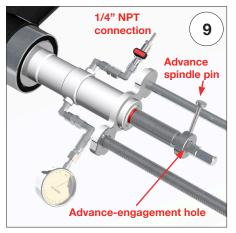
DRILLING SHAFT ENGAGEMENT Line-up first advance-engagement hole available in drilling shaft and re-engage advance spindle pin. BE-FORE TAPPING, leak test the whole new distribution line. 1/4" NPT connection can be used as an inlet port.
