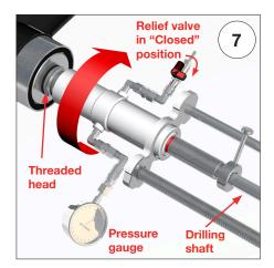
TAPPING TOOL ATTACHMENT Slide it over/onto the drilling shaft and rotate it (clockwise) onto the threaded head of the Supraflow<sup>®</sup> fitting, by hand, until it bottoms out. Attach pressure gauge provided to the quick-connect port and close relief valve.
