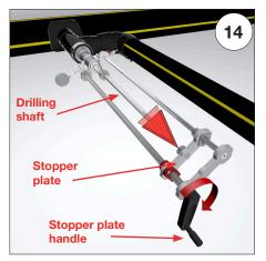
DRILLING SHAFT RETRACTION Rotate stopper plate handle (clockwise) until it bottoms out. Ensure that drilling shaft travels with stopper plate; if pressure is not pushing drilling shaft out, pull it manually until it can no longer be retracted.
